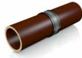
Center coupling over joint. Tighten clamps and shear band reciprocally.
