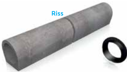
Remove damaged pipe section.
