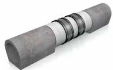
Insert new pipe section and joint with a standard coupling.
