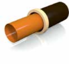
Push pipes together.
