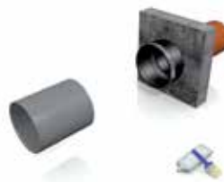
Insert Single Pipe Connector into larger pipe. Apply lubricant to plain ended pipe.
