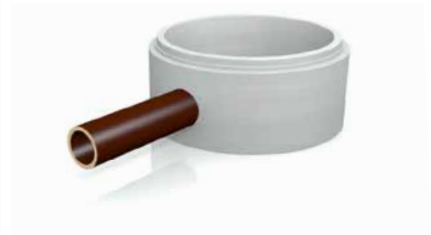
Push pipe into socket.
