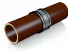
Center coupling over joint. Tighten clamps and shear band reciprocally.
