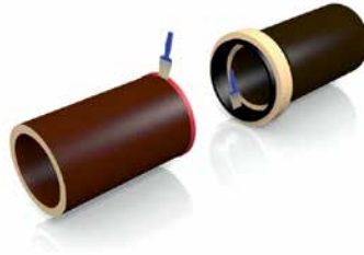
Apply lubricant to socket and M-P-Ring.
