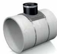
Position T-Flex centrally over cored hole and tighten clamps around the main sewer.
