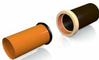
Apply lubricant to socket and Ü-P-Ring.
